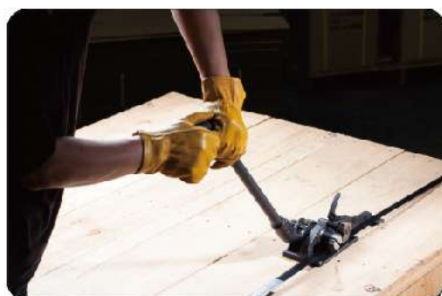
Apply more tension to the strap when needed
