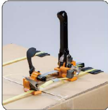
Tighten the strap and insert the seal
