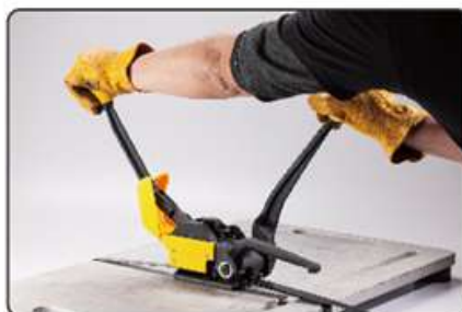
Seal and cut the strap
