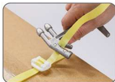
Cut the excess strap
