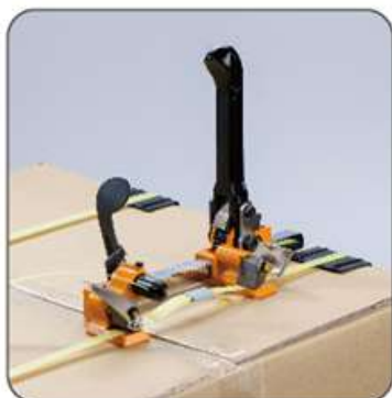
Tighten the strap and insert the seal
