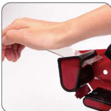
Push the wiper forward to disconnect.
