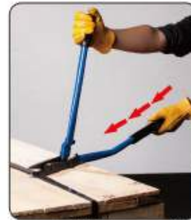
Hammer the blade to squeeze it in between the strap and package.
