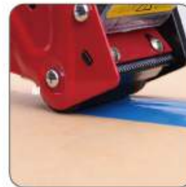
Blade is away from the tape and box when applying tape.
