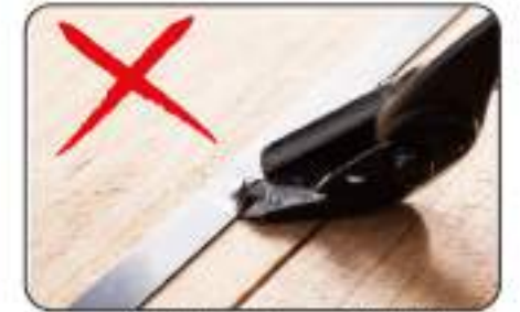
No more twist that damage the blade, strap and/or the package.
